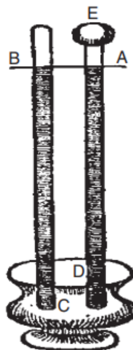
Picture: Torricelli's vacuum experiment in 1644. A and B mercury levels in C and D tubes are equal regardless of the additional volume E in tube D (Jousten, 2016).
